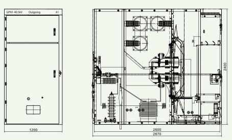
GPN1(C)-40.5 Structure drawing for VD4/VH4 type
