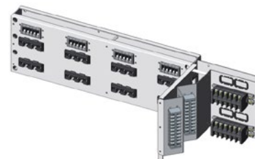
Figure 2 GPJD-6-1/4-32A/3 power distributor side outlet pattern
